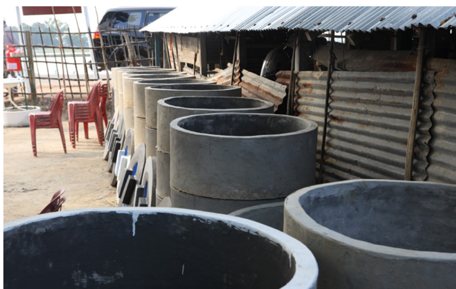
► Figure 12: Latrine rings at a producer centre. The use of saline water reduces the durability of these rings from 5 years to only 6-8 months (Nayeem Khan, 2021:6)
