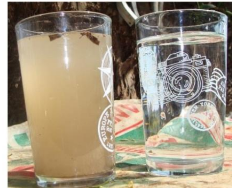
The filtration method tested proved to reduce turbidity levels as well as heavy metal contamination
