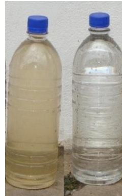
The filtration method tested proved to reduce turbidity levels as well as heavy metal contamination
