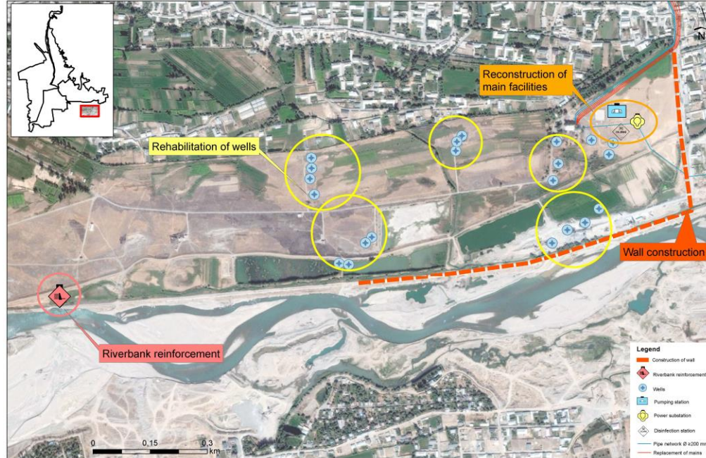
Intervention to the East Part of "KAF-1" Water Intake
