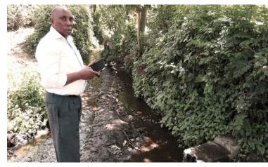
Tito Kitomari taking a discharge measurement with the smart phone app developed by the project (discharge.ch).
