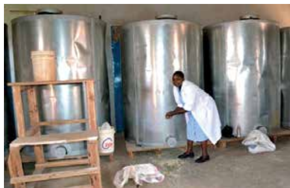
Metal silos at Kamuthatha Boarding Primary School in Embu County, Kenya. The school acquired six 2.7-tonne capacity metal silos and got more benefits than anticipated: reduced postharvest losses (previously amounting to 60% of stored grain); and no need for storage pesticides. The technology helps the school save about US$ 3,600 per year.
