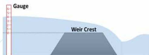
Figure 75: Gauge station at the weir in the secondary canal
